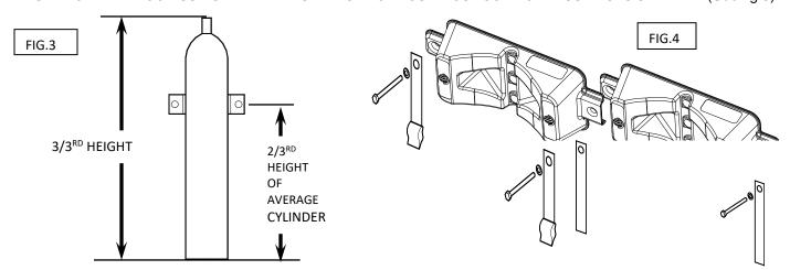
4) PUSH EACH BOLT AND WASHER THROUGH THEIR RESPECTIVE HOLES ON THE UNIVERSAL CYLINDER BRACKET AND PROCEED TO ANCHOR THE UNIT TO THE WALL OR MOUNTING SURFACE. IF MULTIPLE UNITS ARE BEING INSTALLED, THEY WILL OVERLAP AND LOCK TOGETHER WITH THE 2 STRAP ENDS BEING SECURED IN THE OVERLAPPING FLANGE. (See fig.4).
